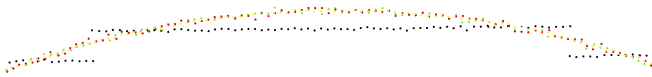
Fig. 10: Comparison of Gazebo and Rmagine LiDAR simulations. Here, a Velodyne VLP-16 was placed 0.5 meters above a virtual ground plane. The image shows a part of the 6th scan line simulated by Gazebo on CPU (yellow), Gazebo on GPU (black), Rmagine with Embree backend (red), and Rmagine with OptiX backend (green).
