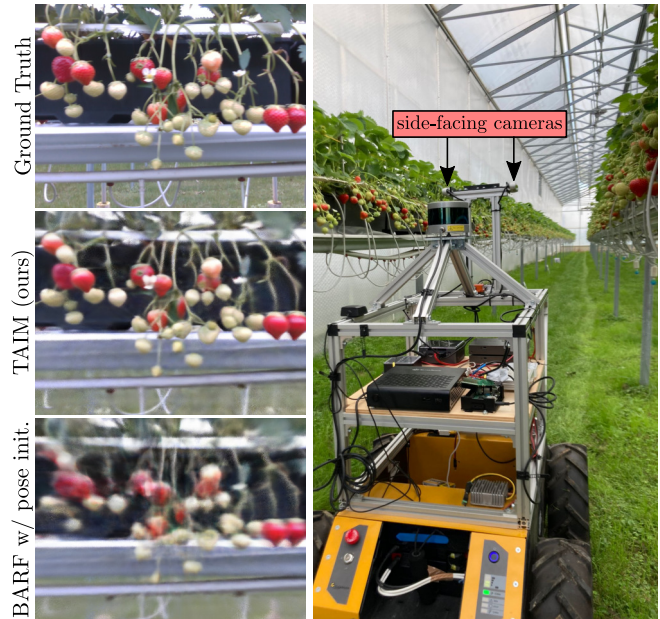
Fig. 1: Right: Our robot capturing images of crop rows inside a greenhouse. Left: Qualitative view synthesis results of our method, TAIM, compared to a baseline, BARF. We achieve higher-fidelity view synthesis, especially on fruit regions of the scene.
