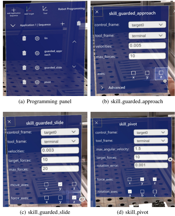
Fig. 5: Programming panel (a) and skill parameter panels (b-d) to set the parameters of the respective skill. Additional expert parameters, e.g. controller gains, are provided by an 'advanced' tab (b).
