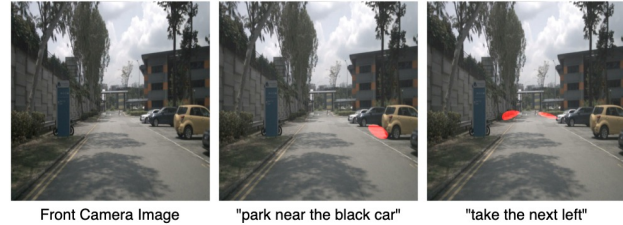
Fig. 1. A major limitation of single image based grounding methods is that they fail if the language command is not immediately visible, which restricts these methods to be used for VLN. Here, we show an example result using the RNR model and on an image from their dataset [4]. The model accurately localizes the black car (middle), however, it completely confuses when asked to predict the left turn, which does not exist in the current view.
