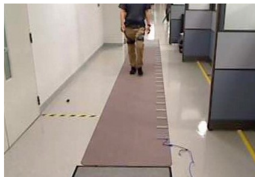
Fig. 6: A subject is walking on a GAITRite system wearing GEMS-H, the hip exoskeleton.
