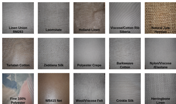
Fig. 5: Physical fabrics. There are 15 kinds of fabrics used in our experiments, which are made of different materials and manufactured using different weaving or knitting methods.
