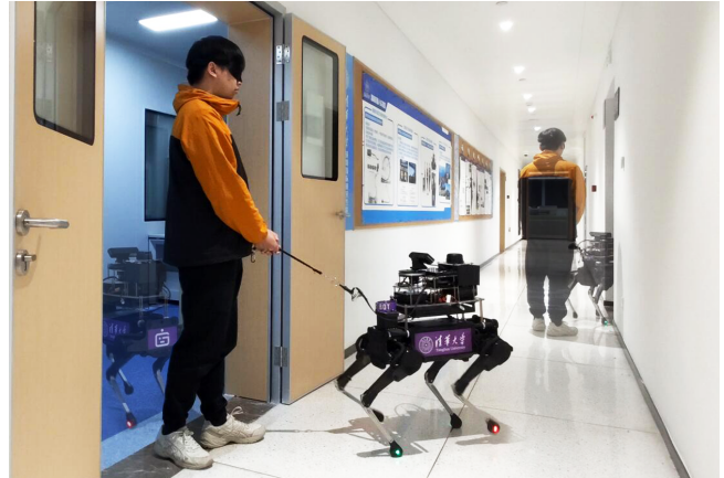
Fig. 1: A blind-folded person is guided by Laikago to turn out and cross the corridor. The person is guided by an elastic rope and a force control device is used to control the force to ensure comfort.
