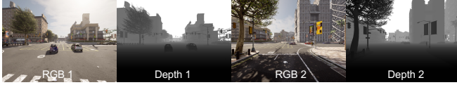
Fig. 4. Examples of the simulated color and depth images obtained by two connected vehicles at the same intersection from different perspectives.
