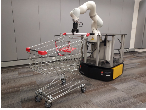
Fig. 7. Mobile Manipulator and shopping cart setup.
