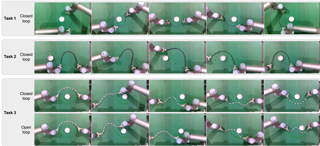
Fig. 6. Manipulation processes of three real-world tasks using the proposed planning and control framework. The green+black circles refer to the final desired DLO configurations. For Task 3, we also show the comparison between the proposed closed-loop manner and the open-loop manner.
