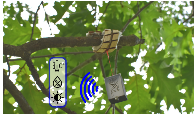
Fig. 1. Biodegradable origami gripper attached to a tree branch. With rain, the gripper degrades and loses its grip, causing the sensor to fall to the ground.
