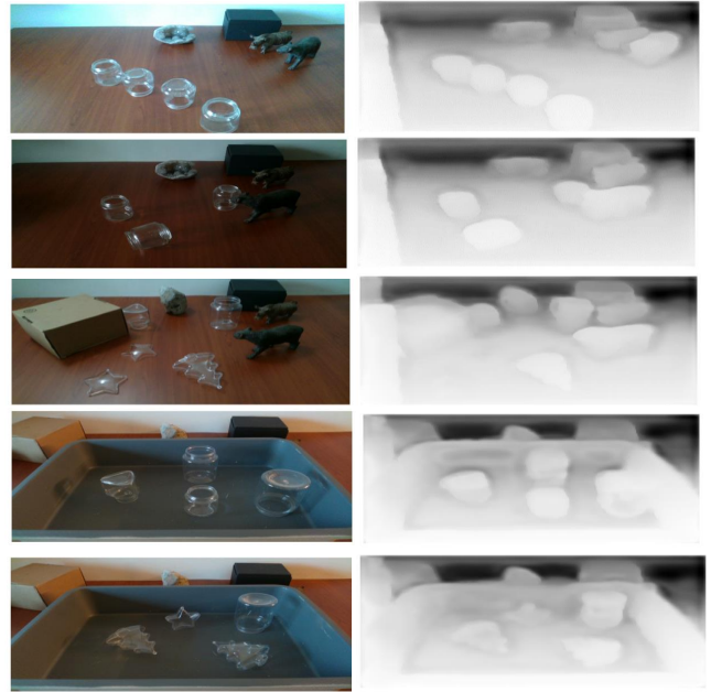
Fig. 3. The samples of predicted depth images from our TODE-Trans model. Under different lighting conditions and scenes, our model provides effective depth prediction for transparent objects.
