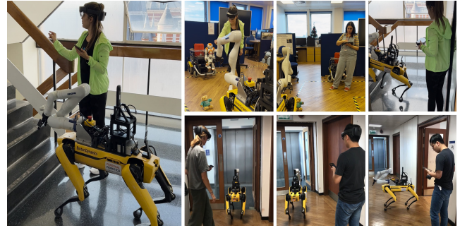
Fig. 1: This paper discusses a multi-dimensional evaluation of our proposed AR HMD UI using validated metrics relevant to a successful human-robot interaction. We compared our AR HMD UI against off-the-shelf hand-held UIs provided by the manufacturers. Moreover, our user study involved navigation and manipulations tasks with varying difficulty levels using a Boston Dynamics' Spot ® , a 7 DoF Kinova ® robot arm, and a Robotiq ® 2F-85 gripper that we integrated into a legged manipulator. See our complementary video.
