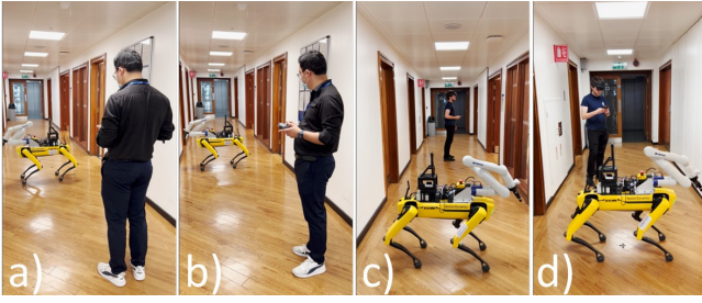
Fig. 8: Cognitive offloading. a,b) When using the controller, some users rotated their bodies to align themselves with the robot and facilitate its positioning. c) We added new functionality to the AR HMD UI that allows the users to position themselves as required. d) After a voice command, the robot will position itself to match the user’s pose. Watch our complementary video for more details.
