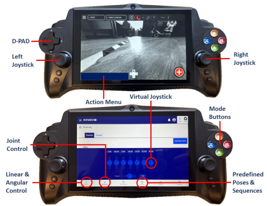
Fig. 2: We used the off-the-shelf UIs developed by BD (top) and Kinova (bottom) to control Spot and the arm from the handheld controller provided by BD with Spot. See Spot controller configurations and Kinova Kortex Web App for further details.
