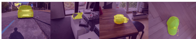
Fig. 3: In some cases, geometry might not get recovered properly, as shown with the hole in the laptop. The hole in the handle of the teapot is not correctly inferred as free space. In the other two cases, some density is assigned outside of the object.
