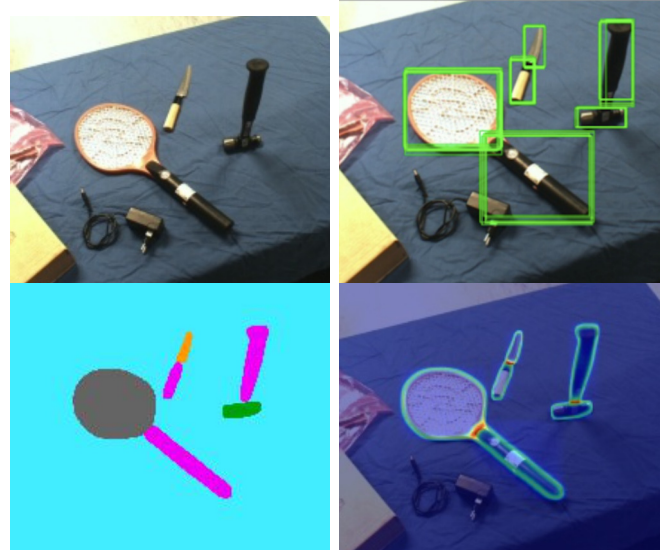
Fig. 1. We detect the affordances in an image (bottom-left) from a RGB image (top-left). Our Bayesian Instance Segmentation architecture produces a probabilistic distribution of the mask and class label, computing the respective epistemic and aleatoric variance. Despite previous approaches that were limited to a probabilistic detection (top-right), our Our Bayesian Instance Segmentation architecture produces per-pixel variance map (bottom-right).
