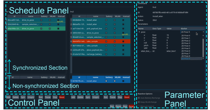
Fig. 6: Screenshot of the command GUI showing a mission for a team of two robots.
