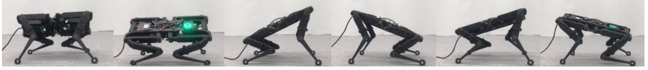
Fig. 1: Snapshots of the first motion scenario (moving the base while balancing, with all feet in contact).
