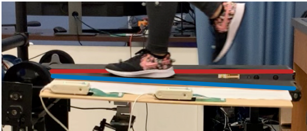
Fig. 3. VST simulating a unilateral low stiffness environment. The left belt (blue) is set to 45 kN/m and the right belt (red) is set to rigid (1 MN/m). As the left leg steps on the compliant belt, the belt deflects vertically due to its reduced stiffness.
