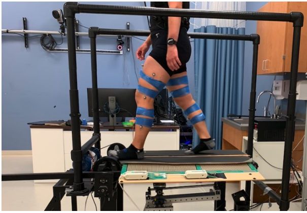
Fig. 2. Subject walking on the VST equipped with electromyographic (EMG) sensors and reflective markers for motion capture. The body weight harness can be partially seen around the subject's torso.
