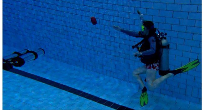
Fig. 1: LoCO AUV running DIP to navigate towards an object in response to diver pointing gesture.
