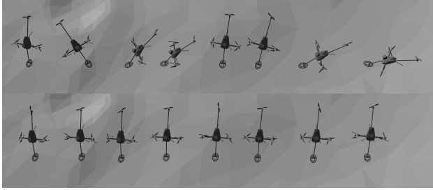
Fig. 6. Irregular, mostly flat simulated terrain. Top : The naive Aligned-1 approach results in inefficient turning. Bottom : With the proposed planner, the system translates along the lane with only slight changes to its yaw.
