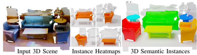
Fig. 1: Mask3D. We train an end-to-end model for 3D semantic instance segmentation on point clouds. Given an input 3D point cloud (left), our Transformer-based model uses an attention mechanism to produce instance heatmaps across all points (center) and directly predicts all semantic object instances in parallel (right).
