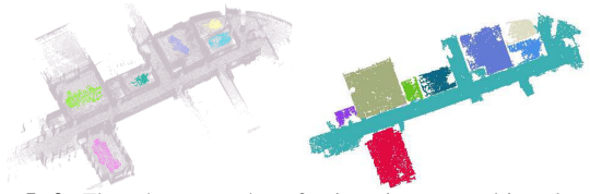
Fig. 5. Left: The robot map where furniture is annotated in color. Right: The robot map after segmentation.
