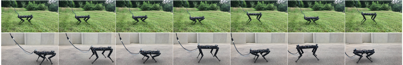
Fig. 1: Solo12 in outdoor experiments. Top: trotting and jumping on grass. Bottom: jumping from right to left on asphalt.
