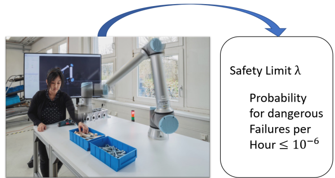
Fig. 1. We present a generalizable method for quantifying the propagated measurement uncertainty (PMU) to evaluate safety limits in robot systems. According to official regulations, we refer to the probability for dangerous failures per hour (PFDH) to distinguish safe from dangerous situations.
