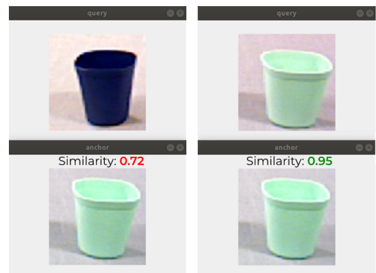
Fig. 8. The siamese similarity comparison; the left vertical pair has a similarity score of 0.72, and the right vertical pair has a similarity score of 0.95. The top query images are in the robot’s view, and the bottom anchor images are in the robot’s long-term memory.
