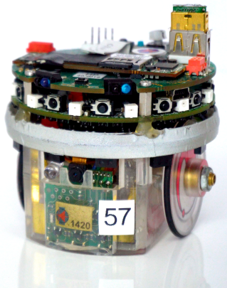
Fig. 1: The e-puck robot and its reference model RM1.1.
