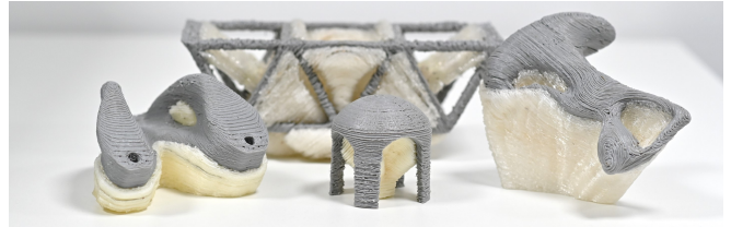
Fig. 9. Example models that have been fabricated by our robotic system – (left) Topo-Opt, (middle) Dome, and (right) Yoga with supporting structures.
