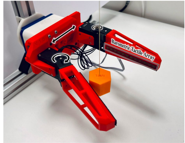
Figure 1: The E-TRoll hand has two rotary joints and a prismatic palm, with a barometric tactile array mounted on one of the two fingers. The orange test object is automatically lifted to the desired height for rolling.
