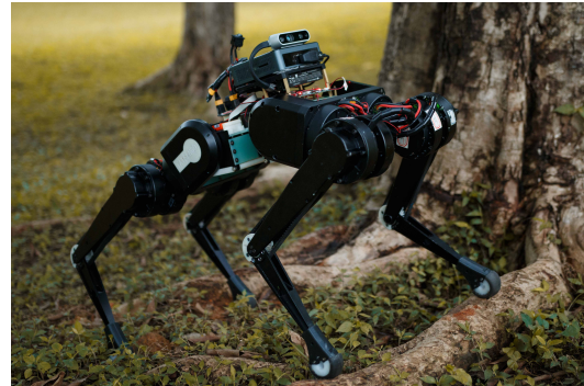
Fig. 1. The Yat-sen Lion quadruped robot platform has 15 actuated DoFs, three per leg and three in the spine.
