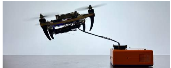
Fig. 2: Un-docking maneuver. AutoCharge ensures universal, highly efficient, and robust charging by combining a portable ground station with a flexible, lightweight charging tether.
