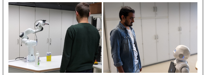
Fig. 1. Human-Robot interaction environments. Left image: pick and place environment with Franka-Emika Panda robot. Right image: pepper robot interacting with a human.
