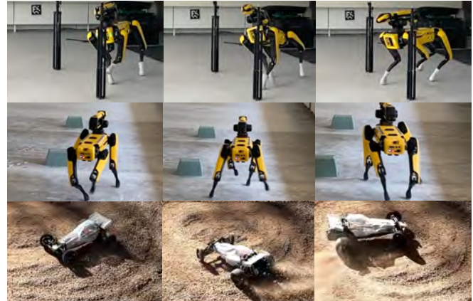
Fig. 1: We evaluate two distinct robots Boston Dynamics Spot and a dynamic RC car. For the Spot, we consider a normal and slippery terrain. We simulate the slippery terrain by using socks at its feet. This causes the spot to slip and lose balance, as depicted on the top three images.
