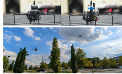
Fig. 1: (Top left) Low-altitude UAV for map refinement. (Top right) high-altitude UAV for aerial mapping. (Bottom) Active metric-semantic mapping by two autonomous UAVs without using GPS.
