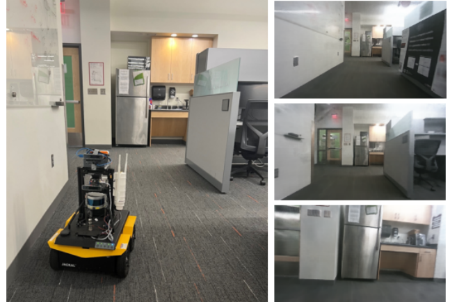
Fig. 1. Real-time experiments with Loc-NeRF using a Clearpath Jackal UGV (left) equipped with a Realsense d455 camera. Examples of NeRF renderings near the beginning, middle, and end of the experiment (right).
