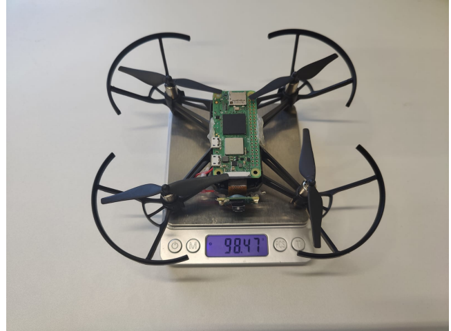
Fig. 1. A DJI’s Tello drone equipped with our Raspberry Pi Zero ver 2 micro-computer, connected to an RGB camera. Our deep learning-based systems are executed on this hardware.
