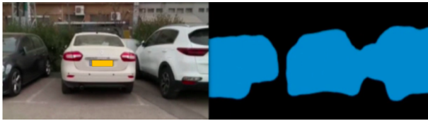
Fig. 3. Left: The original video seen by the drone. Right: The semantic segmentation for detecting empty parking spots
