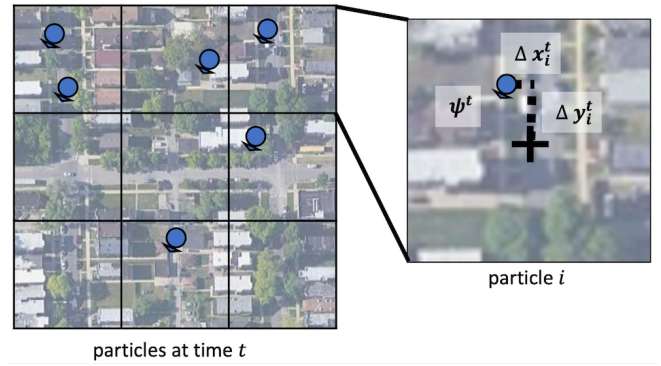
Fig. 4. Particles are dispersed through search area, which is segmented into satellite tiles whose embeddings are precomputed before runtime. At each time step, the true heading of the ground agent is approximately known and the x , y location of each particle within its satellite tile is given by its displacement from the center of the tile.
