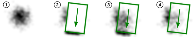
Fig. 3: Spills and crumbs wiping simulator using the SDE in (1) with dirty particles in black and wiped region in green. (1) Initial state. (2) With (\lambda, \alpha) = (0, 0) , we simulate crumbs that are pushed by the wiper. (3) With (\lambda, \alpha) = (0, 0.05) , we simulate a spill that is pushed on a table and sticks below the wiper. (4) With (\lambda, \alpha) = (5, 0.05) , we simulate a spill that is partially absorbed by the wiper.
