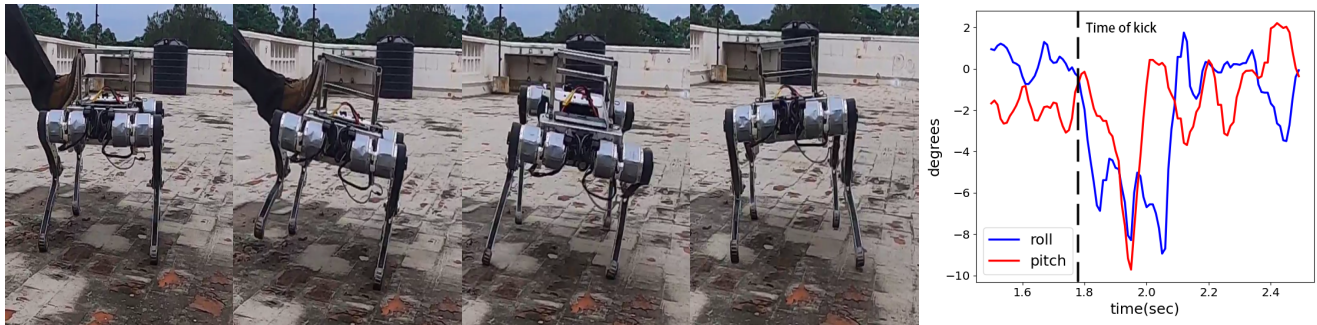
Fig. 6: Stoch3 recovering from external pushes (left), and the corresponding roll-pitch deviations (right)
