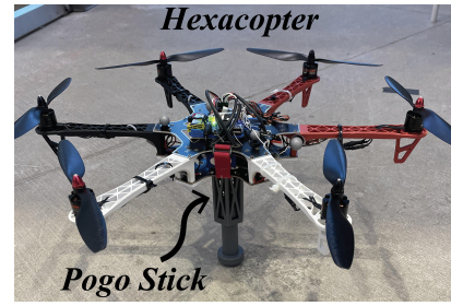
Fig. 6. Modified DJI F550 Hexacopter (550 mm wheelbase) that is acting as the UAS for bouncing interactions. The attached pogo stick was used to facilitate collision.
