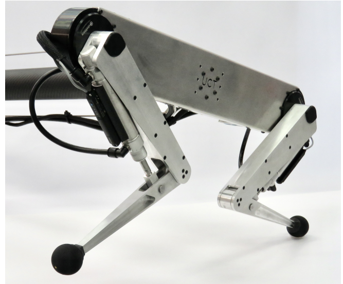
Fig. 1. Kemba , a hybrid electric and pneumatic legged robot designed for rapid maneuvers.
