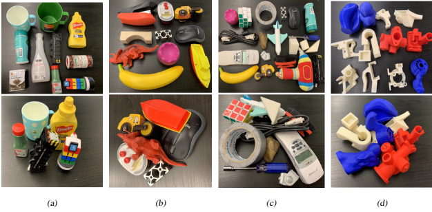
Fig. 5. Object sets and test configurations used for real robot experiments. From left column to right column: packed scene with 10 objects; pile scene with 10 objects; 20 test hard objects [12]; 12 Berkeley adversarial objects [35].
