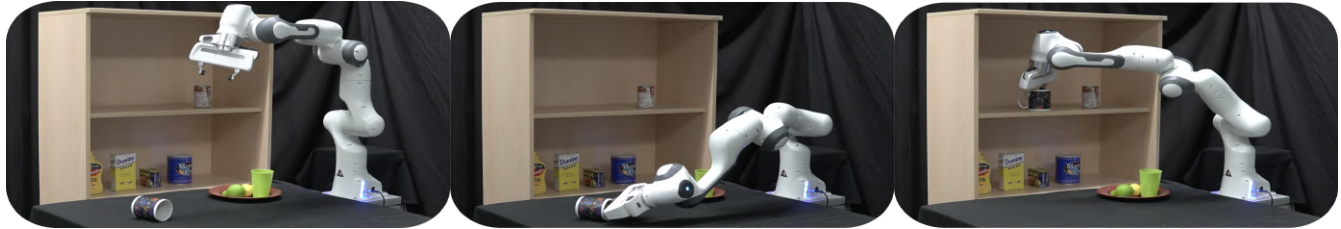
Fig. 1: Pick and place task in which the robot has to pick a mug and move it to the target pose (in the shelves) without colliding. We exploit diffusion models for jointly optimizing both grasp and motion and show the successful trajectory from left to right.
