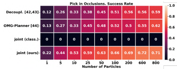
Fig. 5: Evaluation Pick in occlusion. We measure the success rate of 4 different methods based on different number of initializations.
