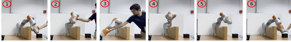
Fig. 3: Obstacle avoidance with external pushes. The image numbers correspond to the time sequence in the key frames.
