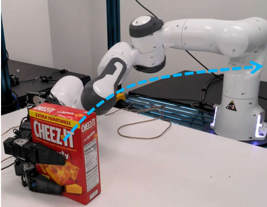
Fig. 5: Picture of our real world task setup. The D’Manus robotic hand is controlled to lift the “Cheez-Itz” cracker-box from YCB [23].
