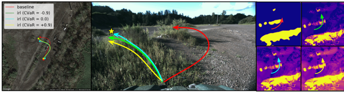
(a) Costmaps learned via IRL allow the robot to cut a corner over some low grass (about 15cm), while the baseline takes a longer route (note that obstacle inflation makes the grass patch appear as an obstacle to the baseline).
