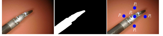
Fig. 3: The Figure shows the original frame, the related binary mask, and the point identification in the image plane.
