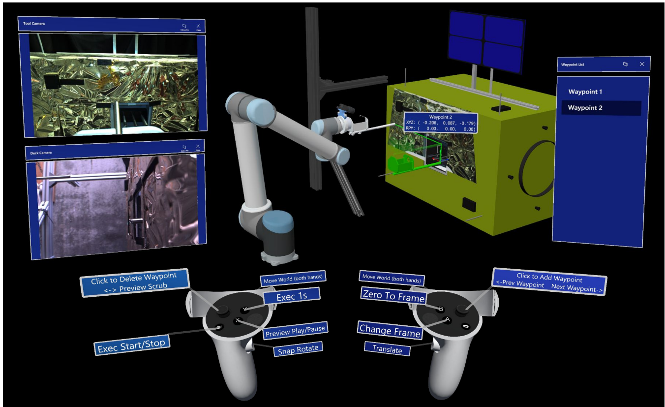
Fig. 4. A screenshot of the operator's perspective in the Meta Quest 2 headset. The 3D virtual planning scene (top center) shows the pose of the space-side robot relative to the satellite and refueling tool station. Operators can place green waypoint markers to create a motion plan using the Meta Quest 2 6-DOF hand controllers, which are displayed virtually with labeled buttons (bottom). Virtual camera windows (top left) display live 2D video from space-side cameras. The waypoint list (top right) displays the waypoints in the motion plan and highlights the currently selected waypoint.
