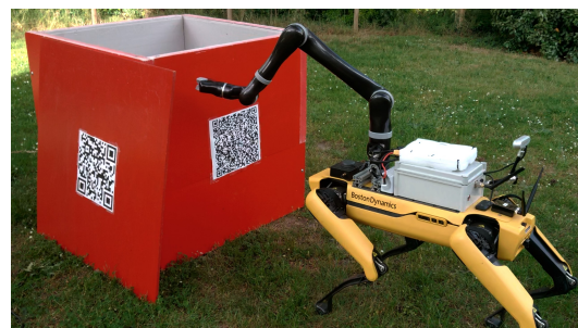
Fig. 1. Spot ® quadruped robot equipped with a Kinova Jaco manipulator arm and a mounted computer executing controller code. The system has to deactivate traps, represented as wooden cubes with a panel that needs to be pushed to neutralize the trap.
