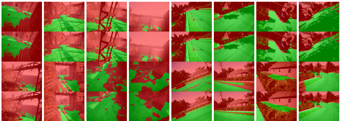
Fig. 7. Qualitative evaluation of our self-supervised traversability labeling proposed in Section III-C compared with the simulated precise traversability labels on TartanAir training sets. The left side is generated from sequence P000 of the abandoned factory environment, and the right side is from sequence P000 in the neighborhood environment. The top two rows are the selected best examples of the generated (first row) and simulated precise (second row) traversability labels, and the bottom two rows show the worst cases in the same order. The color images are overlaid with the labels for visualization.
