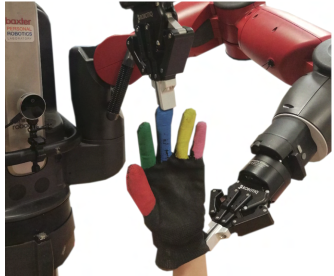
Fig. 1: The proposed method enables the Baxter robot to dress a mannequin’s hand with a glove. Different kinds of alignment action primitives are selected through a high-level rule-based decision process. In the lower level bimanual multisensory control methods are used to align the glove with the hand.
