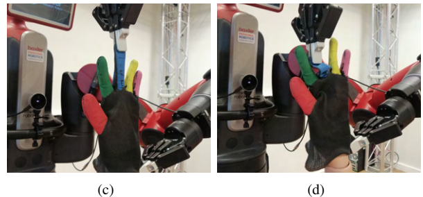
Fig. 5: The visual error (euclidean distance) and the force of the two end-effectors are shown for the hybrid force-vision control (a) and visual servoing (b), while snapshots indicating the behaviour of the two controllers are shown in (c) and (d) respectively. The desired forces of the hybrid controller are set to [0,0,4] and [0,0,-4] for the right and the left arms respectively. The proposed bi-manual force-vision controller manages to maintain the glove under tension and drive the finger’s opening around the fingertip of the hand. Without the force feedback the finger insertion task fails and the robot applies large forces on the hand.
